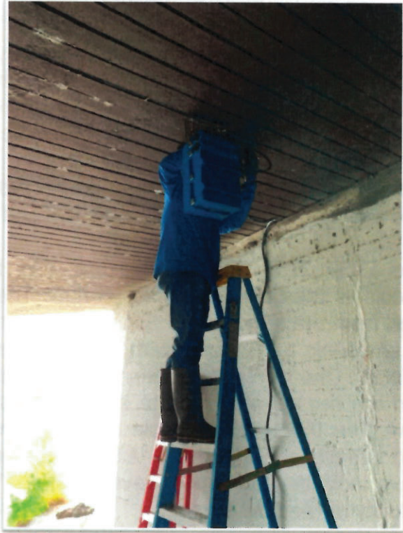
Figures 5a & b: PAS Mounted the ISCO 2150 AV Modules on the Ceiling of RCB and Ran a Flexible Conduit, Along with AV Sensor, Down to the Middle of the Low Flow to Measure the Dry-weather Discharge from Eagle Rock Drain.
