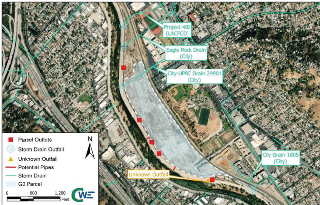
Figure 1-1 Taylor Yard Parcel G2 with Storm Drains
